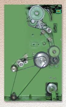
GEAR DRIVE TO TIMER PULLEY CONVERSION Suitable for LR Simplex LF 1400, LF 1400 A
